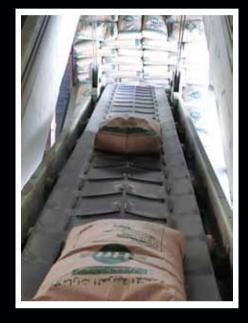
Packing in 3 ply paper bags and 2 ply polypropylene bags of 50 Kg, directly stacked on trucks. The 50 Kg bags are palletized on each pallet 40-50 bags as per requirement of customer.
